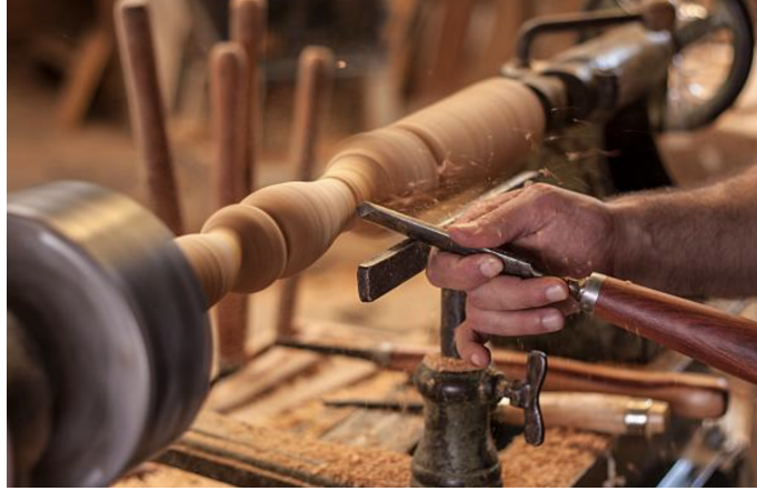
Figure 2: This is a lathe— a block of wood can be carved on it by spinning it and placing tools against it to pick away at small pieces.
